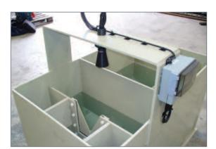
FLOW BOX WITH A V-NOTCH WEIR and dBMACH3
